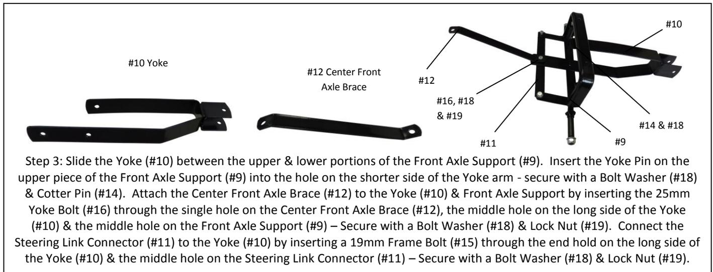
Front Axle Support Assembly (see Steps 2 & 3) – shown with #8 Axle Washers & #7 Axle Cap Nuts
