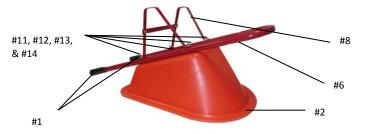
**STEP 3**: Place the Poly Tray (#2) upside down and insert (from the inside of the tray) the Tray Bolts (#9) through the Tray, the Handles and the Leg Assembly. Use Flat Washers (#12), Lock Washers (#13) and Nuts (#14) to secure. Tighten Loosely.
