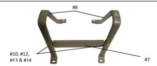
Step 3: Attach the Leg Connector (#7) to the inside of the Legs (#8) by placing Back Leg Bolts (#10) through the legs and the leg connector. Use Washers (#12), Lock Washers (#13) and Nuts (#14) to secure. Tighten Loosely.
