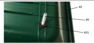
Step 4: Place the Poly Tray (#2) upside down and insert Tray Bolts (#9) through the 4 holes in the bottom of tray from the inside sliding Rubber Washers (#15) over the Tray Bolts (#9) on the outside of tray to hold in place.
