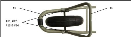
Step 2: Place the Steel Frame/Handles (#1) right side up and attach wheel assembly and front frame support by placing Axle Bracket Bolts (#11) through Front Frame Support (#6), frame & axle brackets on wheel assembly. Use Washers (#12), Lock washers (#13) and Nut (#14) to secure. Tighten Loosely.
