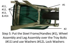
(#13) and Nuts (#14) to secure. Tighten Loosely.
