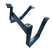
Preassemble the legs (D) by inserting the tab on the brace (E) through the slots in the legs. Lightly tighten the screws (5).
