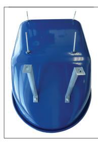
Place tray (A) upside down onto a table or stand. Insert the carriage bolts\* (1, 2) from the inside of the tray through the square tray holes. Rubber washers can be used to hold carriage bolts in place. The long carriage bolts (1) go toward the front. Attach the tray braces (L) to the front of the tray using the short carriage bolts (3). Do not tighten.
