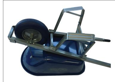
Assemble the wheel by placing the axle (J) through the hub of the wheel. Next place the two axle brackets (I) on the end of the axle. Center the wheel (K) assembly with the axle brackets snug against the hub. Attach the axle brackets with the bolts (4) through the tray braces and handles. Tighten all bolts to complete the assembly.
