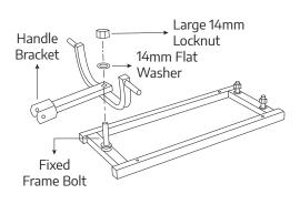
\*NOTE: We recommend to hand tighten all bolts/nuts initially and then fully tighten all bolts with a crescent wrench once full assembly is complete.
